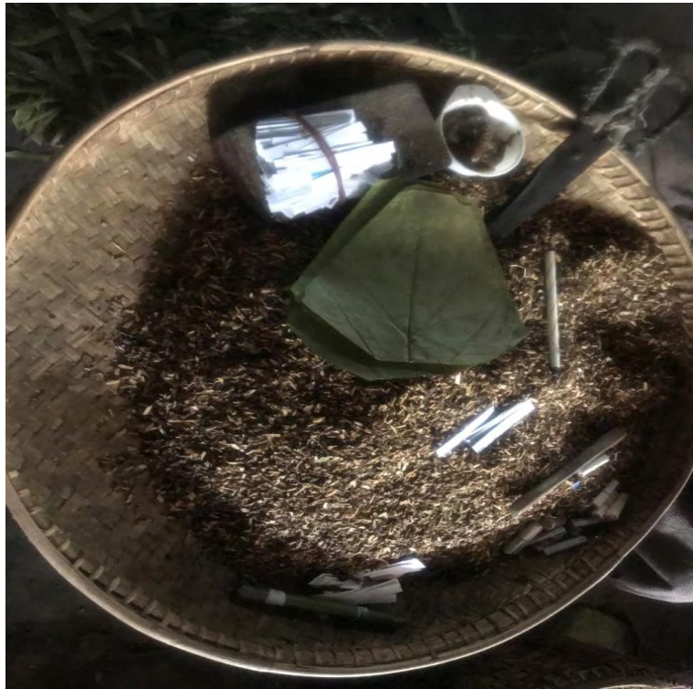
Photo 5: Basic materials for rolling cheroots in a tray (a mixture of processed tobacco, dried tobacco leave-stalks, wooden chips and other combustible materials, added with flavours and additives, ready-made cut filters made with rolled corn leaves, thanatphet leaves, labels, and rolling equipment).
